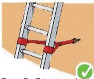
Figure 7 - Tying near the base of the ladder
